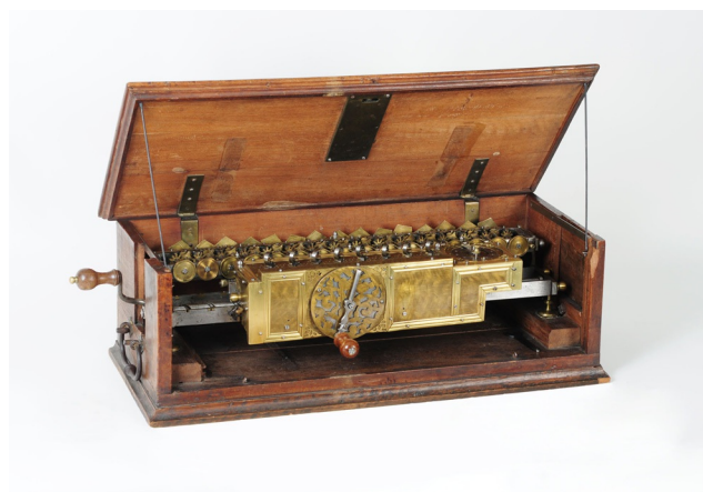
Figure 10. A replica of the Stepped Reckoner, Instrumentum Arithmeticum of Leibniz (original is in the Gottfried Wilhelm Leibniz Bibliothek, Niedersächsische Landesbibliothek, Hannover , image reproduced by permission).
