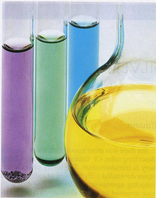
Figure 1. Distinctive colors reveal the oxidation states of vanadium (V) in certain aqueous solutions: V^{+2} (violet), V^{+3} (green), V^{+4} (blue) and V^{+5} (yellow). But there is more to oxidation chemistry than meets the eye.
